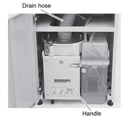
If processing waste remains in the drain hose aperture, clean off the processing waste. If processing waste is not cleaned off, water leakage may result.
