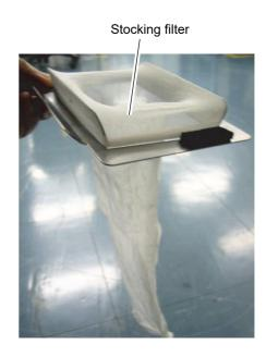
3) While holding the upper flange, first put the stocking filter into the tank and then insert the stocking filter holder into the tank positioned as in the figure to the right.
