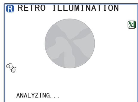
When analysis is complete, the opacity indexes for the center (COI. H, COI. A) and periphery (POI) and a circle indicating the 3 mm range in diameter are displayed.
