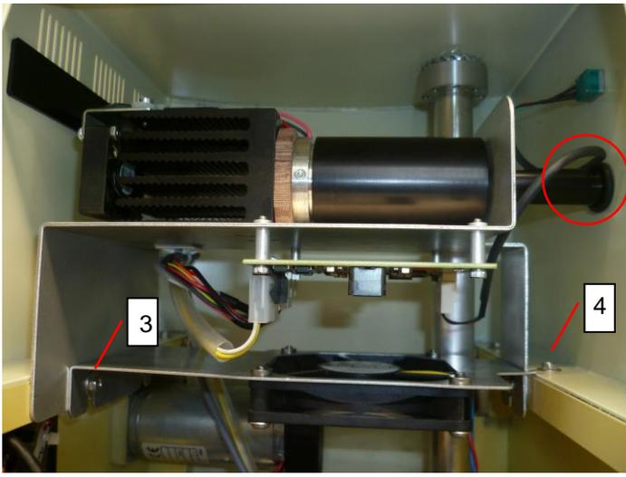
12. Loosen the screw on the left [3] and completely remove the screw on the right [4]. Now the LED module can be pulled out.
