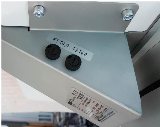
Figure 14 Fuse replacement; fuses F1 and F2.
