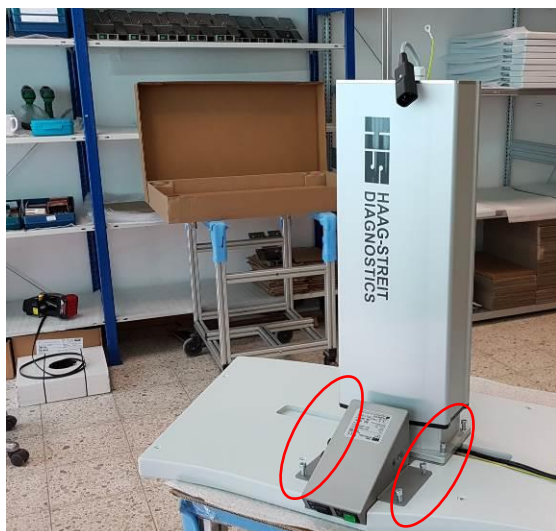
Figure 6 Connection column; fixing the column with 8 screws.
