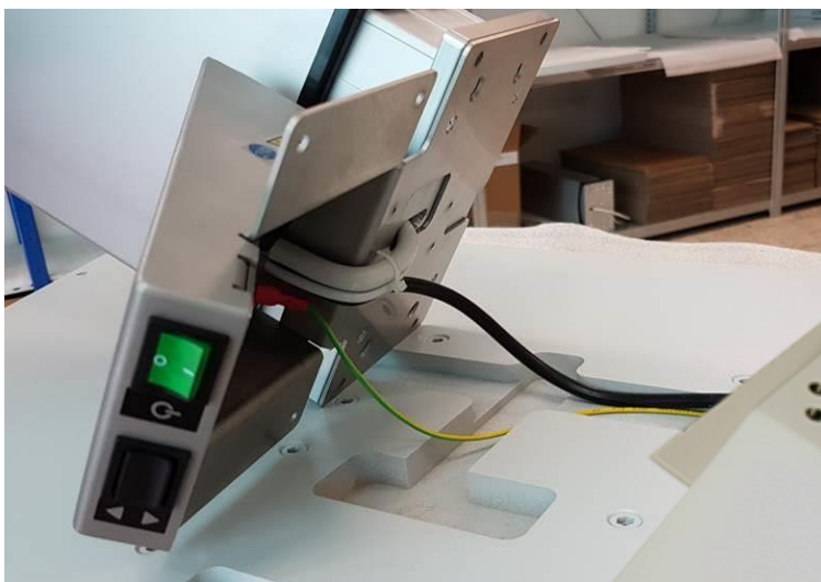
Figure 3 Connecting the lifting column; mounting the cable whip and the earthing cable.
