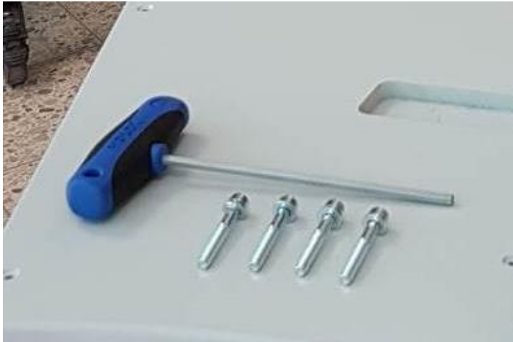
Figure 7 Mounting the Base Plate; preparation.
