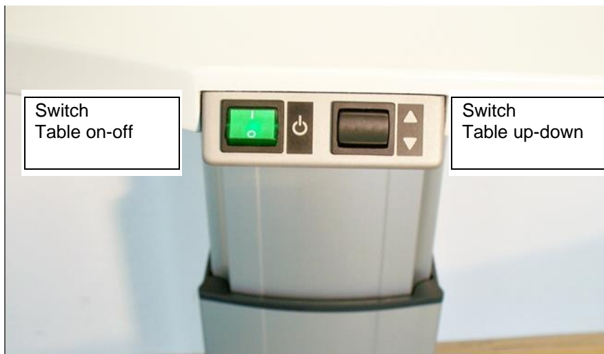
Figure 13 Operating the HSM600 Rocker and toggle switch (operator side)
