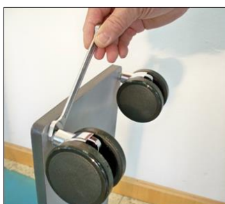
Figure 10 Leveling HSM 600 Instrument table.
