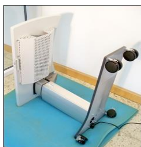
Figure 10 Leveling HSM 600 Instrument table.
