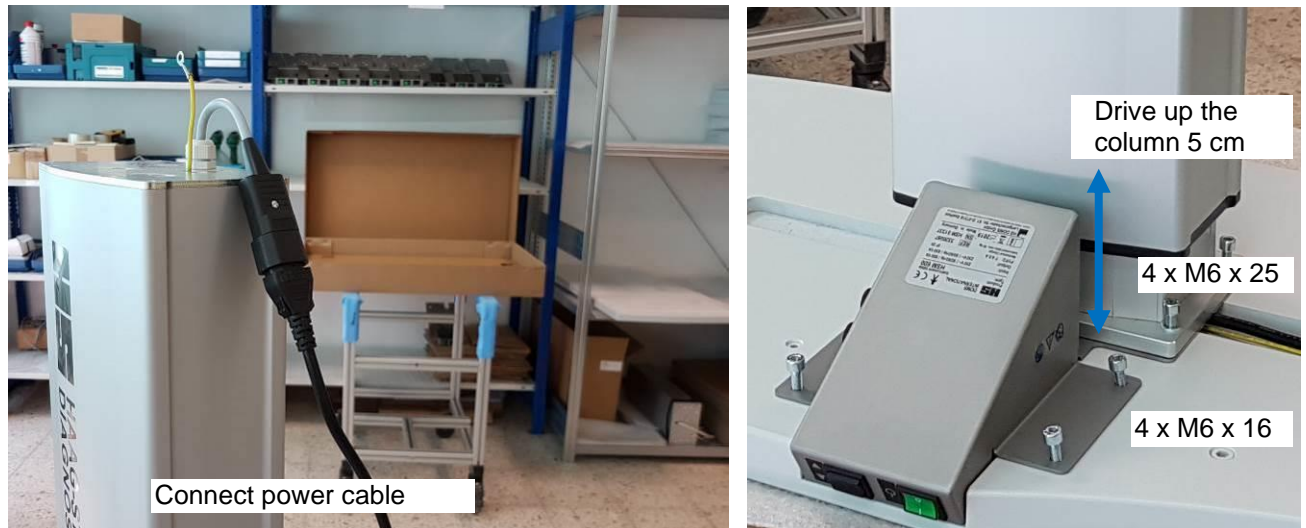
Figure 5 Connection column; connection power cable and mounting column.
