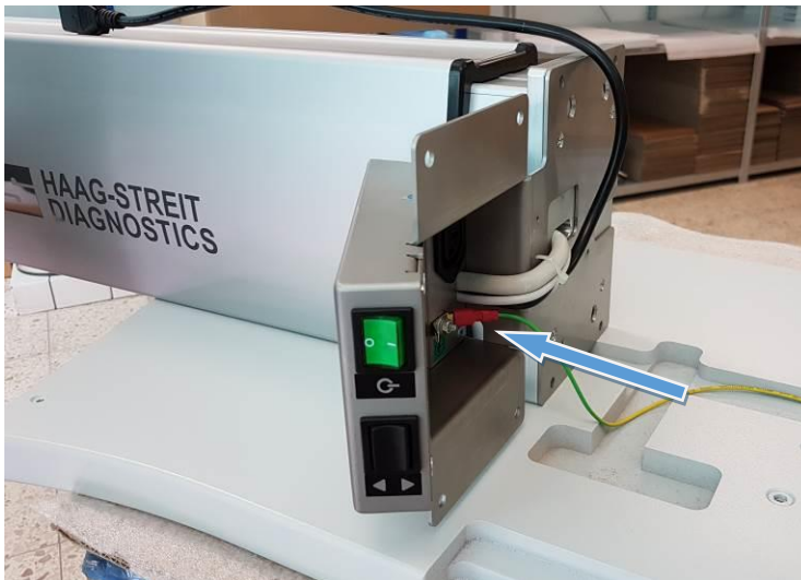
Figure 2 Connecting lifting column; connect earthing cable, secure cable with cable tie.
