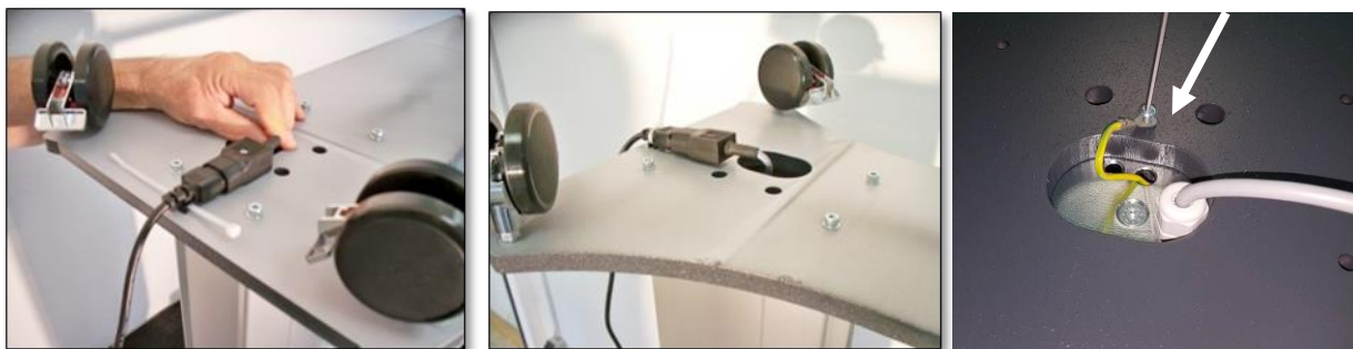
Figure 9 Mounting the base plate; wiring and securing with cable ties.
