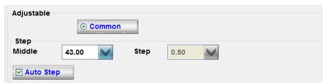
Select the Step setting value from each drop-down list. The setting values on the list vary depending on the selected unit (D or mm).
