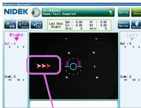
The measuring unit is too far to the left from the patient's eye. Tilt the joystick to the right to move the measuring unit to the right.
