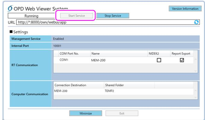
**2** After the service status changes to “Running”, press the Minimize button to hide the OPD Web Viewer System management window.
