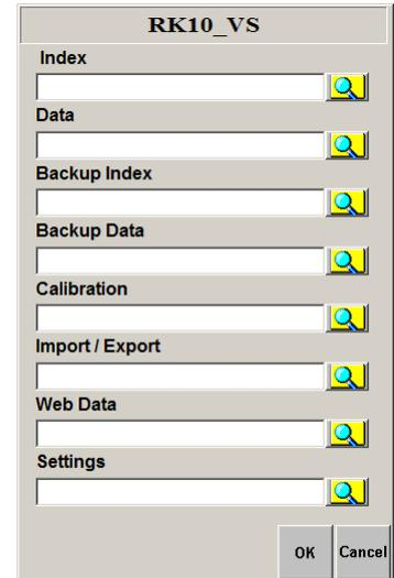
**8** Using the hardware keyboard, enter the target folder name in each field from “Index” to “Settings” in which the database is to be created.
