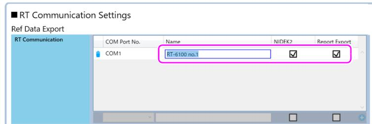
A COM port cannot be edited. To change a COM port on the list, delete the COM port to be changed, then add the desired one to the list.
