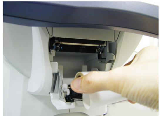
**CAUTION** • When replacing printer paper, be sure not to touch the printer head on the upper part inside printer cover.
