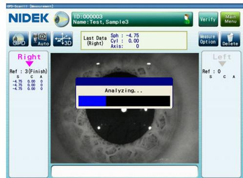
When the OPD measurement is executed for a specified number of times, “(Finish)” appears on the side of number of measurements for “Ref”, and the OPD measurement is complete.
