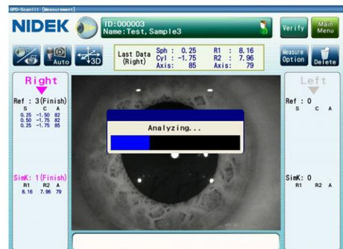
When the CT measurement is executed for a specified number of times, “(Finish)” appears on the side of number of measurements for “SimK”, and the CT measurement is complete.
