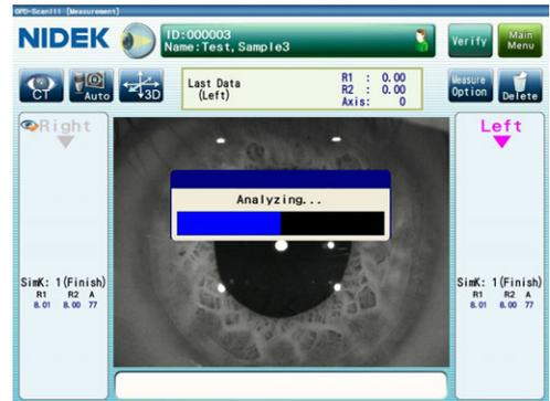
**7** When “(Finish)” is indicated for the CT measurement (SimK), the Verify Examination Quality screen is displayed. Verify the result of image capture and ring edge detection.
