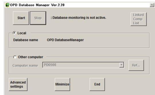
**3** Press the Advanced settings button in the lower left of the screen to display the screen in advanced settings mode.
