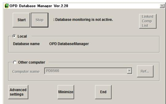
**3** Press the Advanced settings button to display the screen in advanced settings mode.
