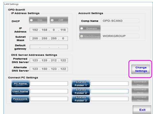
**2** To enable setting, press the Change Settings button. When the message as shown to the right is displayed, press the OK button.
