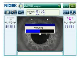
7 When "Finish" is indicated for the OPD measurement, the Verify Examination Quality screen is displayed. Verify the result of image capture.
