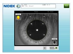
4 Check that the yellow line is placed properly along the pupil edge. If the line is not placed properly, click the button to enter Edge Edit mode.
