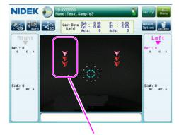
The measuring unit is too high from the patient's eye. Move the measuring unit down.
