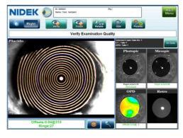
When the OPD and CT measurements for an eye is complete in Single measurement mode, the Verify Examination Quality screen is displayed.
