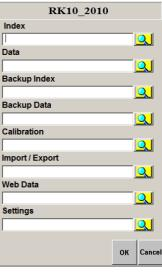
**8** Using the keyboard, input the target folder name in each box from "Index" to "Settings" in which the database is to be created.
