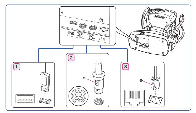
Connect the cable with the device on its side. Ensure that the plug is inserted into the connector in the proper orientation.
