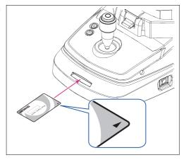
Confirm that the Eye Care card is properly inserted by referring to the Eye Care card icon (EyeC) on the screen.
