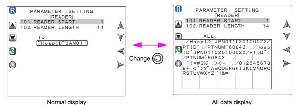
Pressing the change button displays all data including digits other than the set digits. Pressing the change button again returns to the original display.
