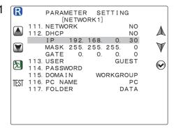
**2** Press the enter button to display the IP address setting screen.
