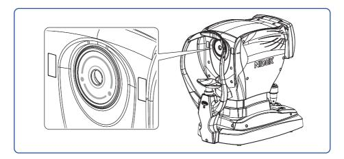
**2** Wrap lens cleaning paper around a thin stick such as a chopstick (or cotton swab) and wipe the lens of the measuring window with a material moistened with alcohol.
