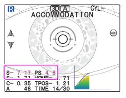
Once measurement starts, AR-measured values and the pupil size are successively displayed along with the graph. When measurement is complete, a beep sounds and the screen display stops updating.
