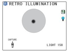
To change the light intensity manually, press the lamp button. As the light intensity automatic control is deactivated, change the light intensity with the displayed up button or down button.
