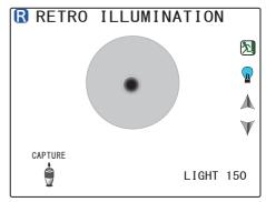
**2** Manipulate the joystick so that the opacity is in focus and the corneal luminous spot is not prominent, and then press the start button for image capture.
