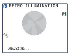
When analysis is complete, the opacity indexes for the center (COI. H, COI. A) and periphery (POI) and a circle indicating the 3 mm range in diameter are displayed.
