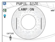
When measuring the pupil size under reduced lighting, turn off the chart-illuminating lamp in the measuring window.
