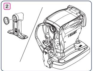
**2** Remove the cap from the spherical model eye and put the model eye on the chinrest with its lens toward the measuring window and then insert the fixing pins.
