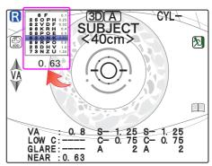
**4** To finish near visual acuity measurement without any addition power (ADD), switch the eye to be measured and measure the other eye in the same manner.
