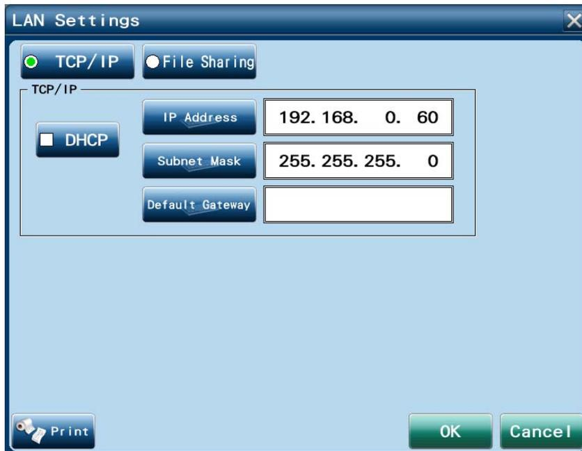
Settings for the IP address and subnet mask of the AL-Scan
