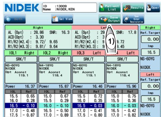
To calculate again after saving, printing, or outputting the calculated result without proceeding to the patient information screen, press the Save Output Recalculation button instead of the Save Output button.
