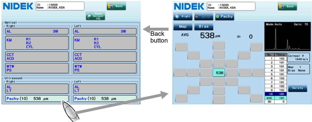
Pressing the Back button in the measured result details screen returns to its original screen.
