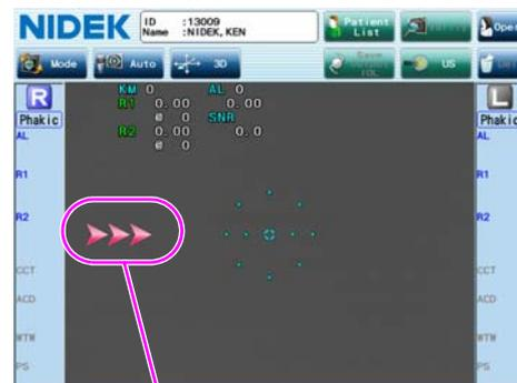
The measuring unit is too far to the left from the patient's eye. Tilt the joystick to the right to move the measuring unit to the right.
