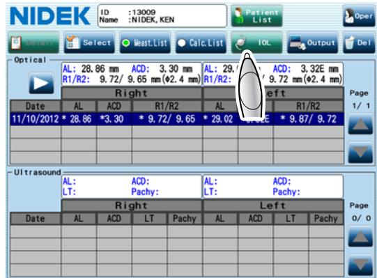
(D) When recalculating the IOL power that has already been calculated, press the Calc.List button in the result screen to display the result screen for IOL calculation. Then press the IOL button.
