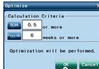
When changing the calculation condition, enter the desired value using the numeric keypad window that appears by pressing the BCVA or Post-Op button.
