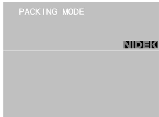
**3** After the screen to the right is displayed, and the main unit and chinrest stop moving down, turn off (○) the device.
