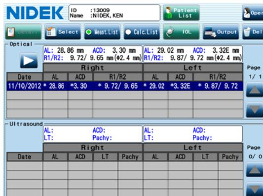
To check the measured result of CCT, WTW, and PS, press the button to toggle the display of the optical measurement result list.
