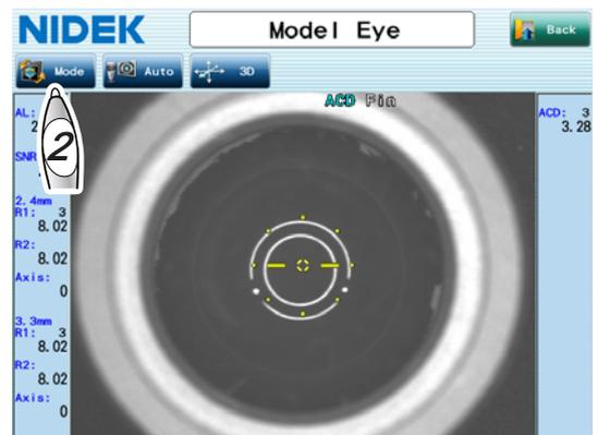
**3** Select the Pachy button in the Measurement Mode window, then press the OK button.
