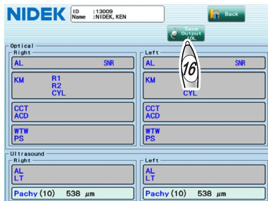
The measured data is saved, and also output or printed depending on the setting. The IOL power calculation screen appears. Go to “2.8 Calculation of IOL Power” (page 90).
