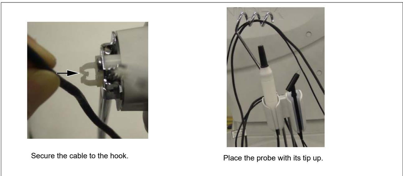
Secure the cable to the hook.
