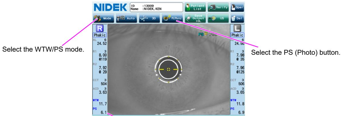
If the pupil size is measured for both PS (Meso) and PS (Photo), the measured value for PS (Meso) is displayed in the PS fields.
