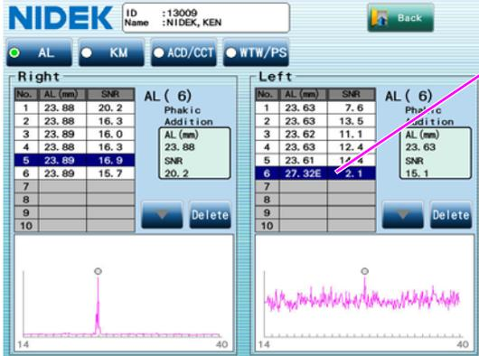
Selecting a measured value on the list displays in purple the waveform from which the value was calculated.
