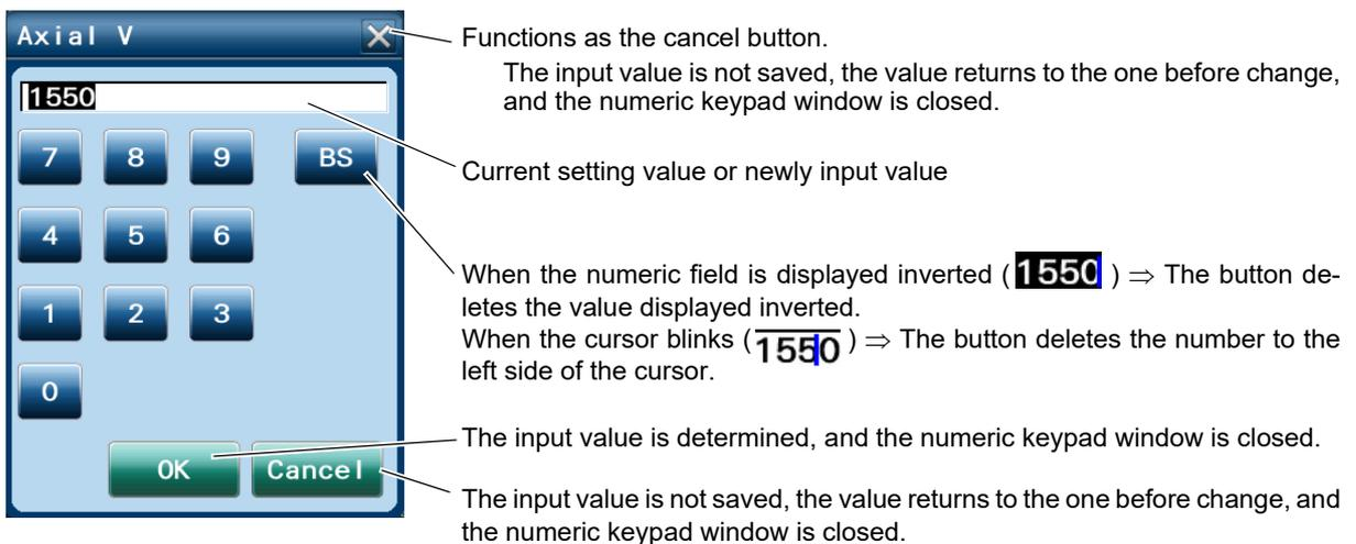
\*Some keys in the numeric keypad window are different depending on the input item.
