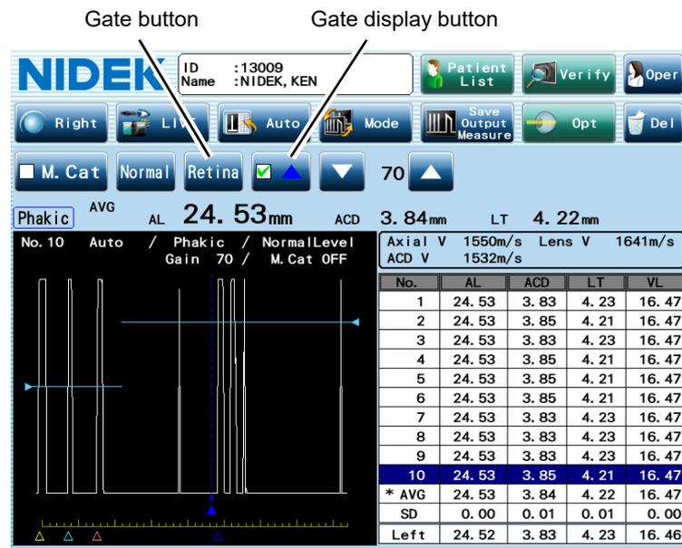
**1** In the BIO mode screen, confirm that no improper A-scan waveform or intraocular biometry values are found.
