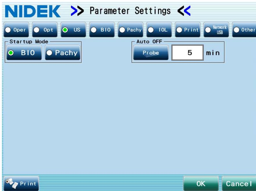
This tab is for the AL-Scan equipped with the optional ultrasonic measurement function only.
