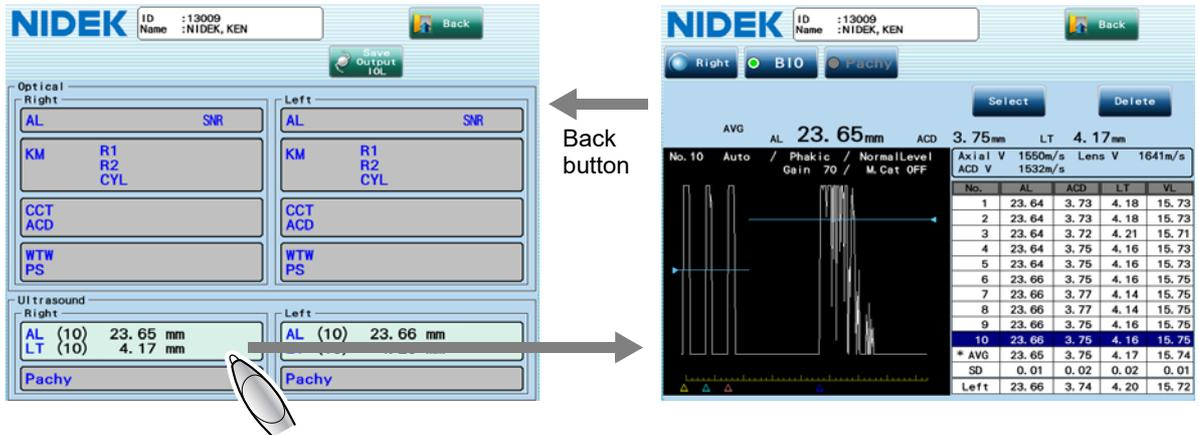
Pressing the Back button in the measured result details screen returns to its original screen.
