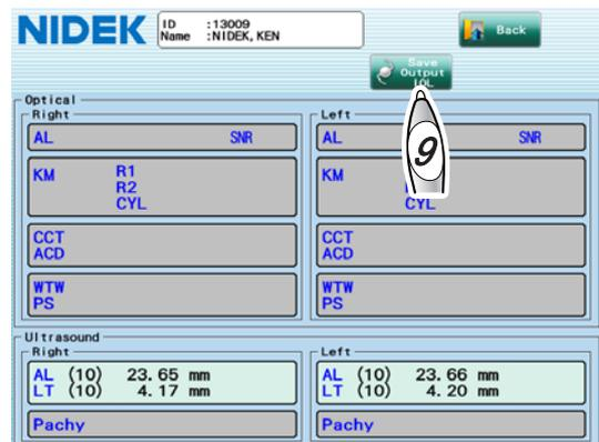
**9 Check the measured results and press the Save Output IOL button to save the measured data, then proceed to IOL calculation.**
