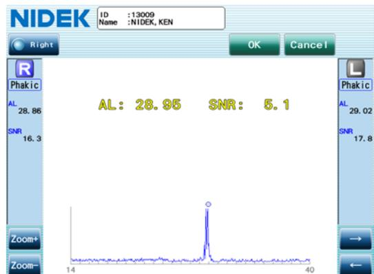
If there are multiple peaks close to each other, enlarge the waveform horizontally using the “Zoom+” button to more easily specify the proper position. Pressing the “Zoom-” button reduces the waveform horizontally.
