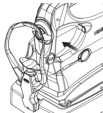
**4** Attach the magnetic forehead rest pad to the system main body.
