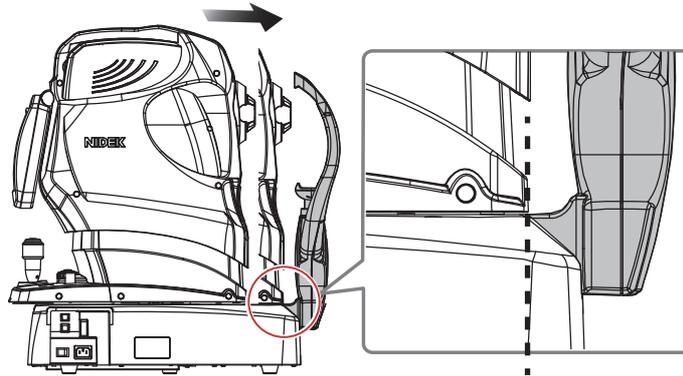
3) If the main unit stops halfway, press and hold the safety stopper, then move the main unit to the edge of the base unit.
