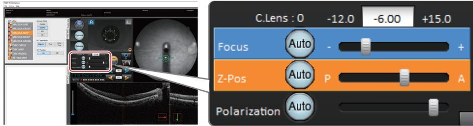
3) If the SSI is low, or the optimization is interrupted, individually adjust the focus, Z position, and polarization.
