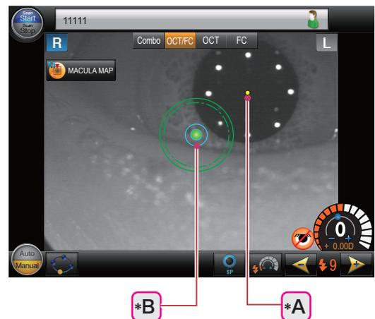
\*1. Factory setting. The standard mode offers a simple screen configuration more specialized in screening than the Professional operation mode, without items such as the OCT Phase Fundus image, scan line, and Z position adjustment button.
