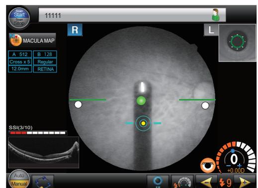
**8** To capture images of other parts, press the fundus image to move the internal fixation lamp.
