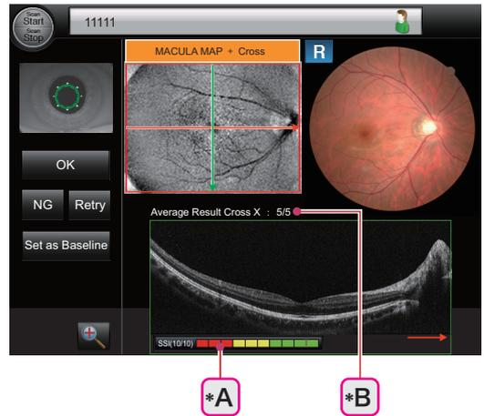
In addition to the images, check the SSI (\*A) and image averaging result (\*B) to evaluate the quality of the OCT image.
