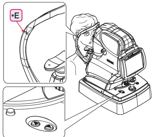
If the limit indicator (\*F) appears in the touch screen of the system main body, move the chin-rest in the indicated direction.
