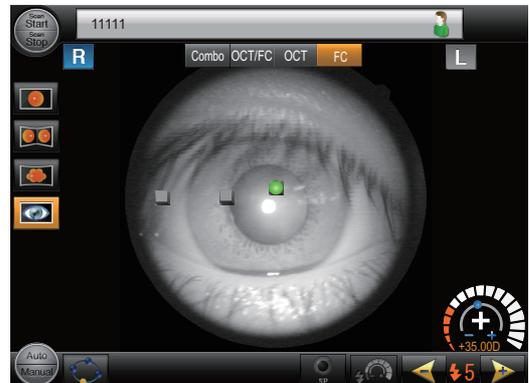
**4** Manipulate the joystick forward and backward to display the eye clearly.
