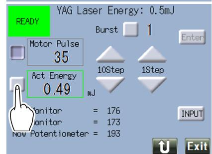
6) Enter the measurement value after the calibration.
