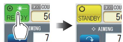
**7** Press the AIMING button to turn off the aiming beam.
