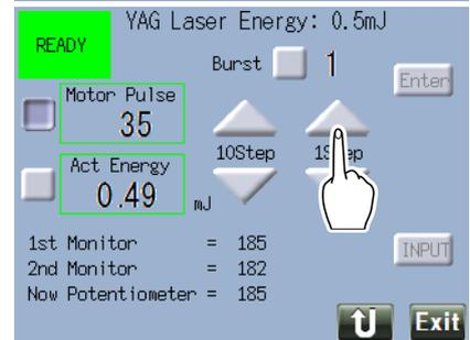
7) Press [Input] to save the parameters for “Motor Pulse” and “Act Energy”.
