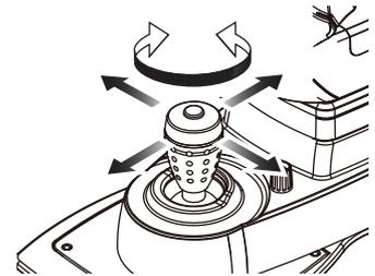
2) Adjust the intensity of the illumination light by turning the illumination control.
