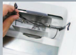
Composite tracing measures the FPD/DBL and frame wrap angle along with the frame shape, thus, calculating all frame measurements automatically.
