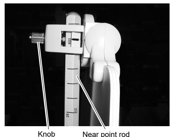
**6** Attach the near point rod in the refractor head.
