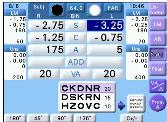
**11** Perform the binocular balance test.
