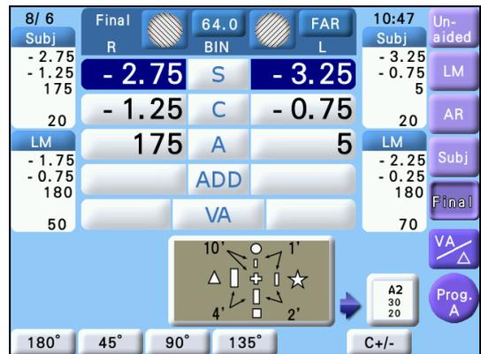
When the patient has stereoscopic vision with a high accuracy (normally 1') and has no symptoms of headache or eye strain, his/her phoria is usually negligible. When the patient can recognize the stereoscopic difference between the top and right lines, his/her stereoparallax is 1'. In this case, it is considered that the phoria test is skipped.
