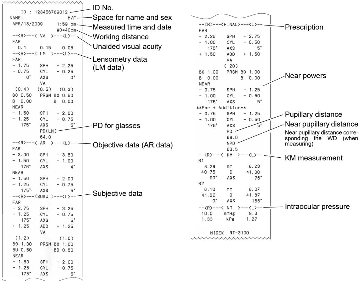
The image shows two sample printouts from a NIDEK RT-3100 device. The left printout contains patient information, working distance, unaided visual acuity, lensometry data (LM data), PD for glasses, objective data (AR data), and subjective data. The right printout contains prescription data, near powers, pupillary distance, near pupillary distance, KM measurement, and intraocular pressure. Labels with arrows point to specific fields in both printouts.
