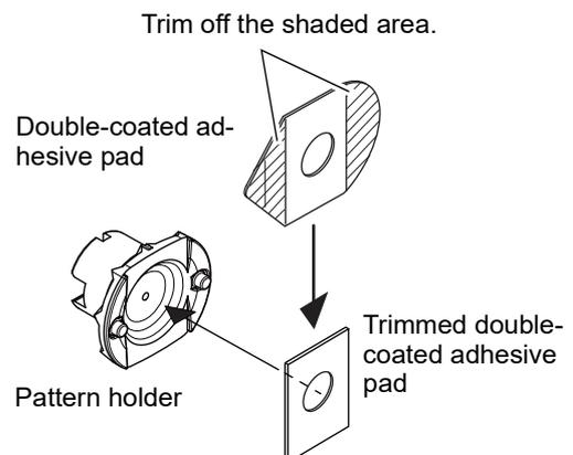
**5** Attach the pattern holder to the calibration jig in the orientation shown to the right.
