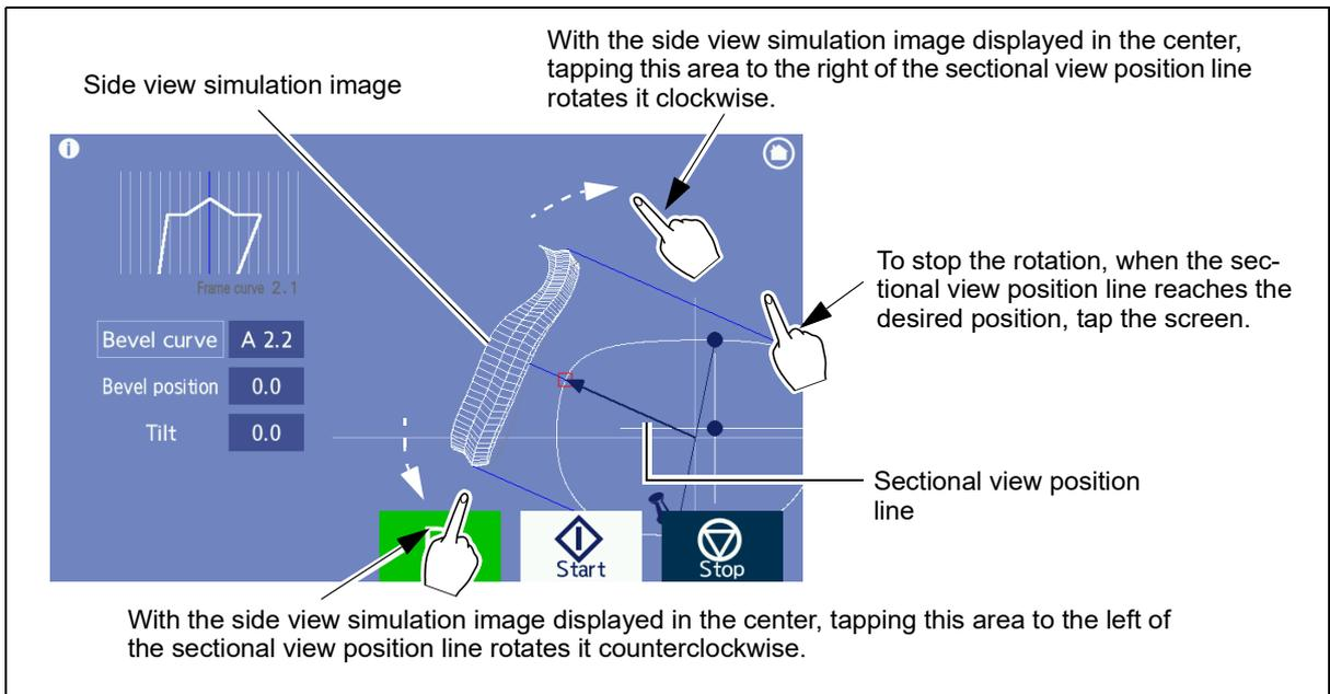
**11** Rotate the sectional view position line and check the bevel sectional view at each position in the sectional view simulation.
