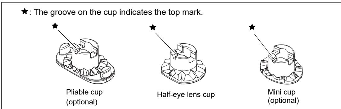
When using the half-eye lens cup, use the double-coated adhesive pad for half-eye lens cup.
