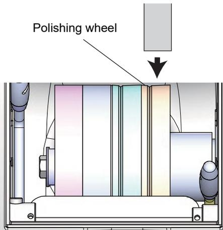
4) When the water begins running again, release the dressing stick from the wheel and wash the wheel surface and dressing stick with the running water.
