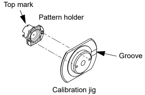
**6** Set the calibration jig to the lens adapter.
