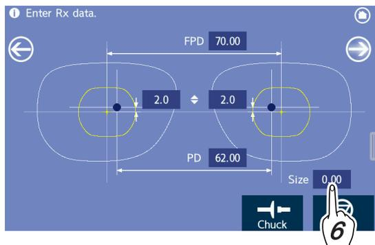
With the entered value, the lens shape is enlarged or reduced on the basis of the shape center while a similar form is maintained.
