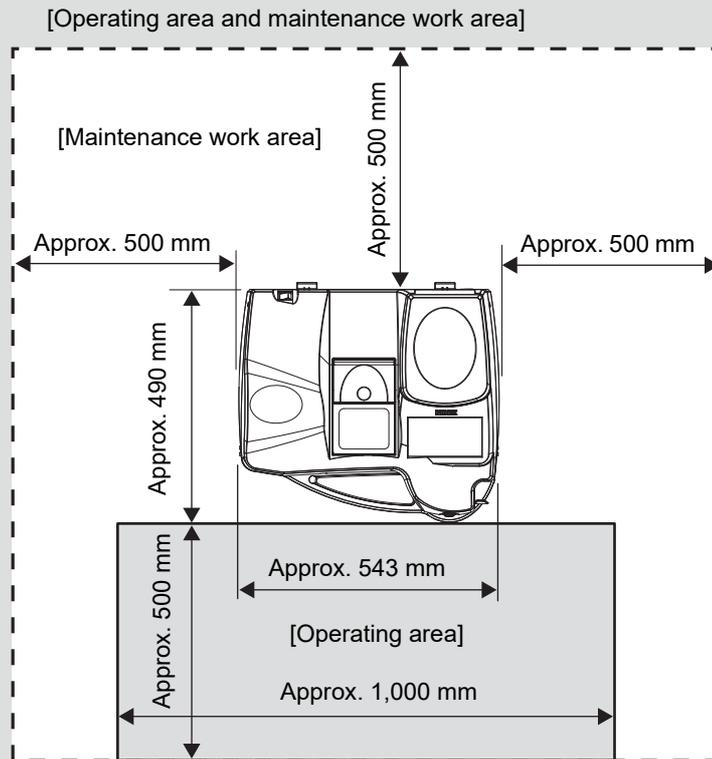
\*As a maintenance work area, a height of approx. 750 mm needs to be available from the level of the table on which the instrument is placed.
