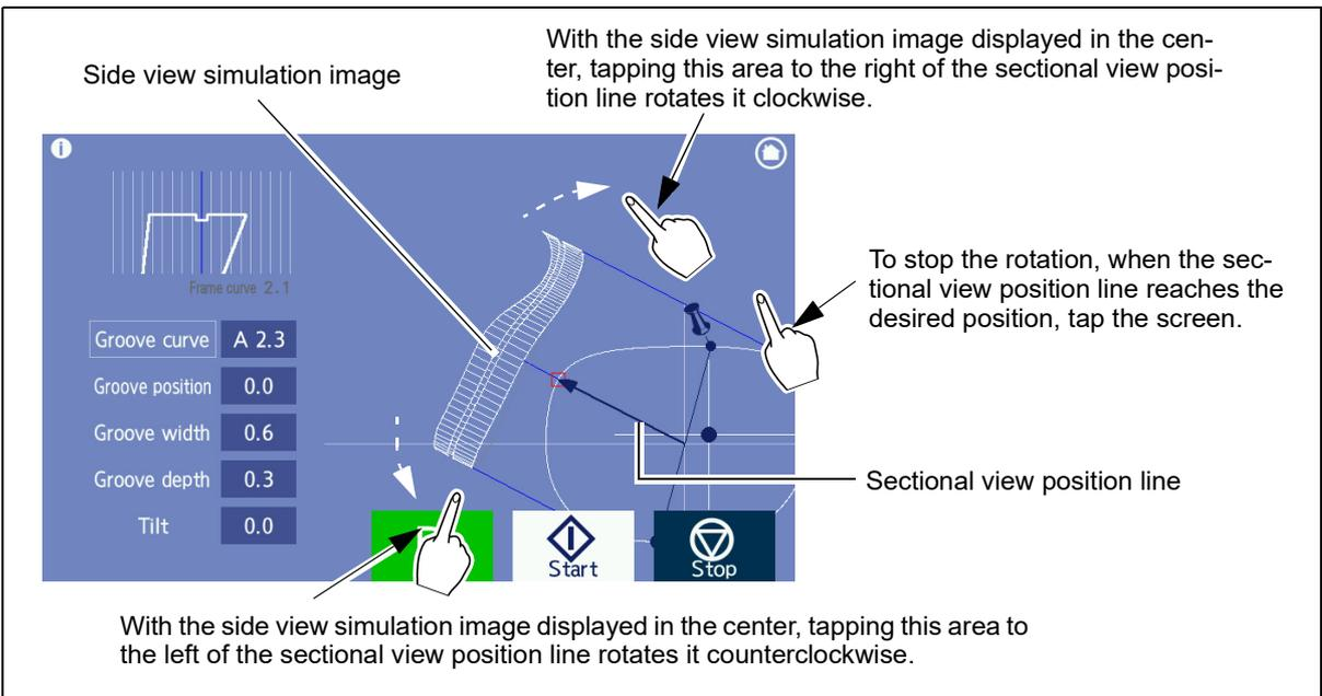
**11** Rotate the sectional view position line and check the groove sectional view at each position in the sectional view simulation.
