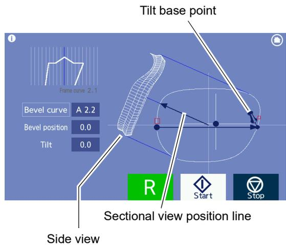
The sectional view simulation of around the tilt base point is displayed.
