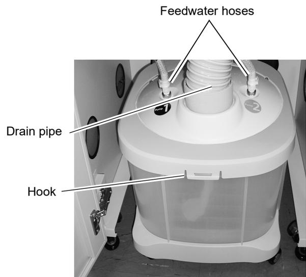
**7** Dispose of the processing waste remaining in the tank as industrial waste. Dried processing waste can be disposed of as general industrial waste.
