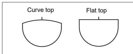
When this parameter is set to "Received" and the "Ethernet port" parameter is set to "VCA-B" or "VCA-C", the segment type switches between "Curve top" and "Flat top" in accordance with instructions from the server.
