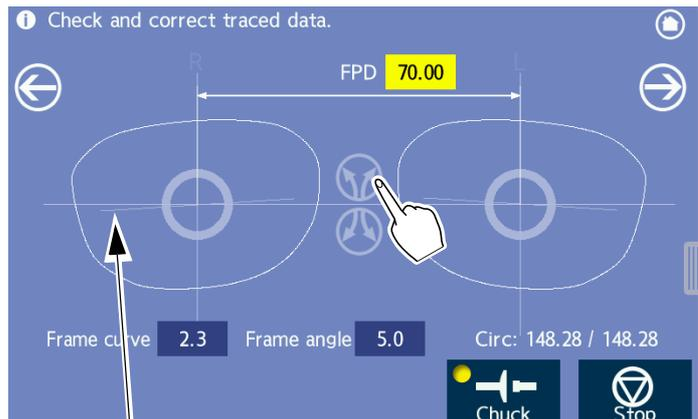
After the axis of the lens shape is adjusted, an axis line is displayed to show the amount of incline from the initial horizontal line. When this line or the circle in the center of the lens shape disappears, the adjusted angle and original angle are in agreement. When FPD or DBL is entered or the screen is changed, this indication is reset.
