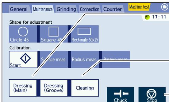
“Dressing (Main)” button: The wheels rotate. Water runs over the wheels for several seconds and pauses for about 10 seconds. The process is then repeated.
