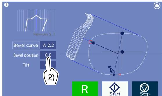
**Ex.—** Entering “-0.4” with the numeric keypad → “←0.4” is displayed in the “Bevel position” numeric field and the bevel position moves 0.4 mm toward the front surface.
