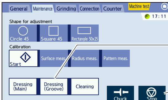
“Dressing (Groove)” button: The grooving wheel rotates at a low speed. Water runs over the wheels for several seconds and pauses for about 10 seconds. The process is then repeated.
