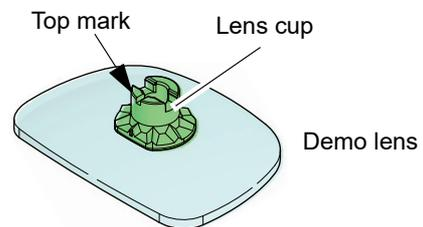
**5** Open the processing chamber cover and set the demo lens to the lens adapter.
