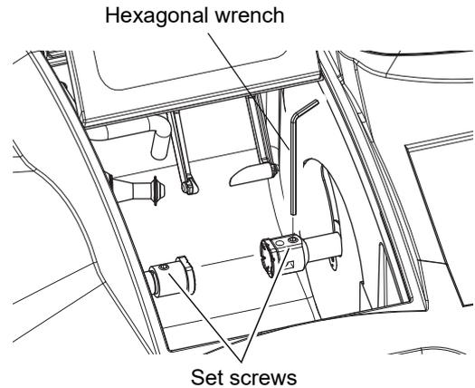
**2** Attach the lens adapter and lens clamp for the mini cup.
