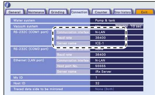
**11** Connect the ICE-1 and LT-980 with the RS-232C cable provided with the LT-980.**12** Turn on the LT-980.
